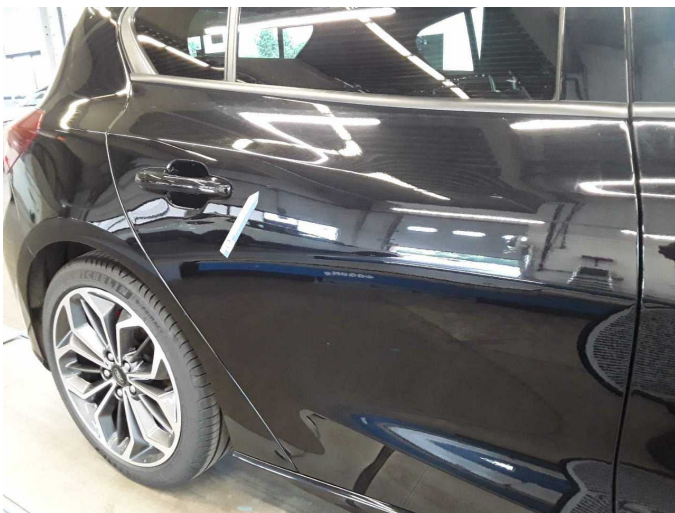
Damage 8: Door - rear right side: Door - Dent / paintcoat damage - Repair and paint
