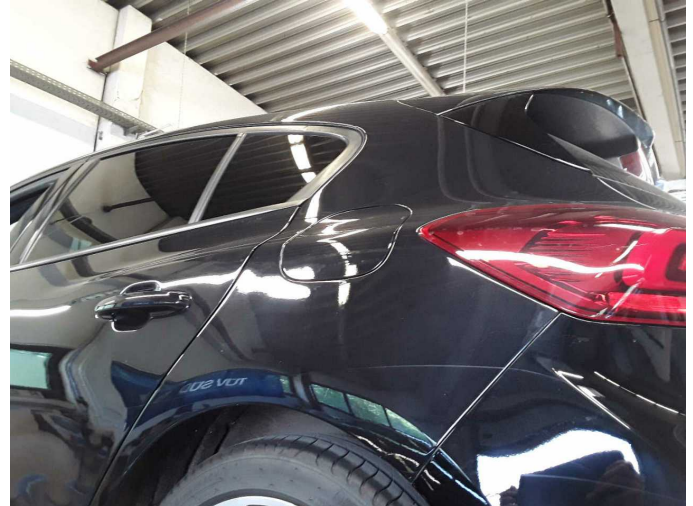
Repainting 1: Side panel - rear left side, Door - rear left side, Door - front left side
