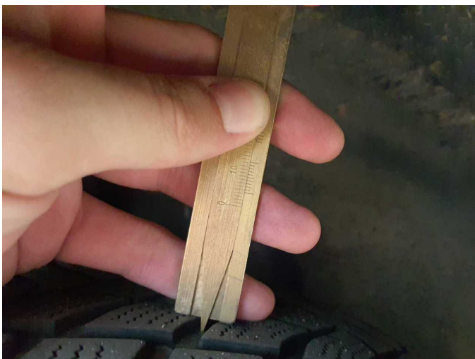
Wear and tear 1: Wheel / tyres: Tyre - rear right side (Über 4mm) - No deduction
