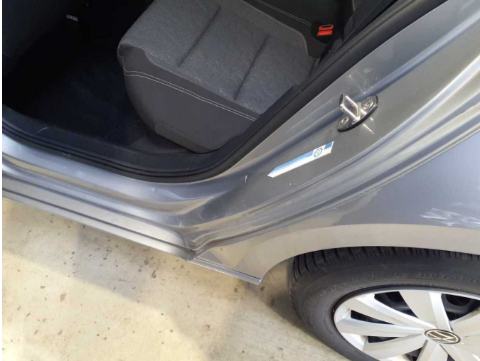
Damage 12: Side panel - rear left side: Sill - Dent / paintcoat damage - Smart repair
