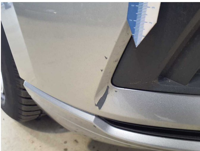
Damage 20: Front bumper: Front bumper - Scratched - Paint
