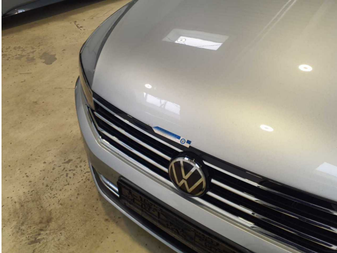
Damage 21: Bonnet: Bonnet (Wellig) - Unprofessionally repaired - Repair and paint
