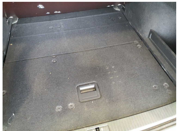
Damage 16: Interior: Cargo area floor - Deformed - Replace
