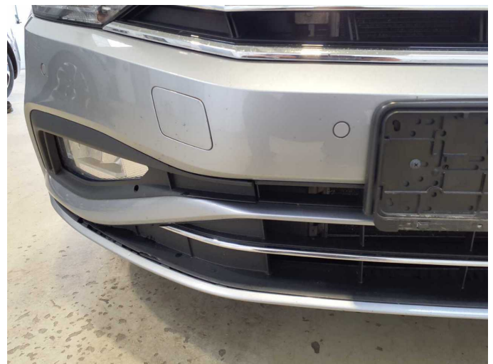
Damage 3: Front bumper: Cover bumper - front - Malposition - Perform diagnosis
