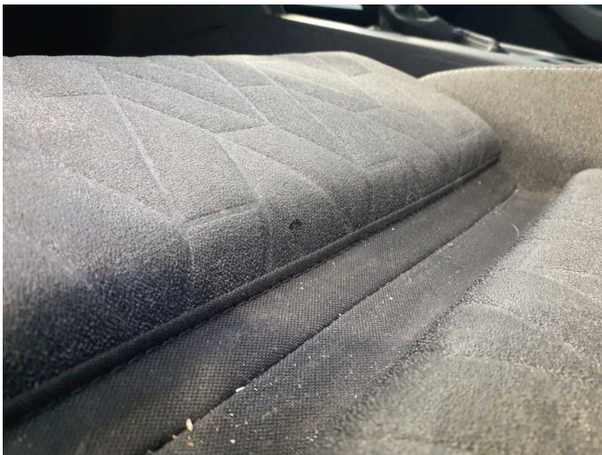
Damage 19: Seat - front: Seat cover - left side - Damaged - Replace
