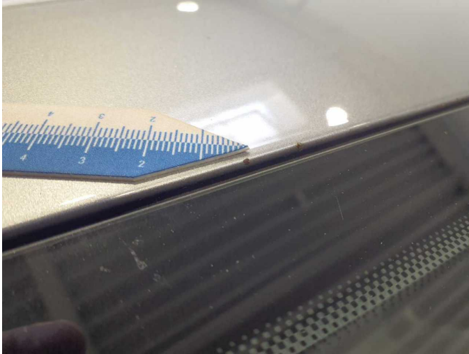
Damage 22: Roof: Roof (Korrosion) - Dent / paintcoat damage - Repair and paint
