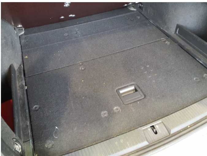
Damage 16: Interior: Cargo area floor - Deformed - Replace
