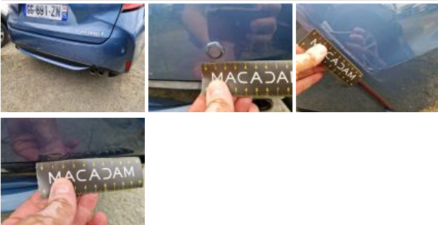
Bumper R, Deformed / Strained, Paint
