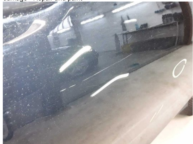
Damage #17: Door - front right side: Door - Dent / paintcoat damage - Repair and paint
