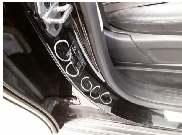
Damage #8: Sill - right side: Sill - Dent / paintcoat damage - Repair and paint
