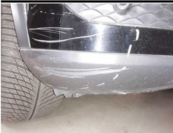
Damage #10: Front bumper: Spoiler - Scratched - Replace
