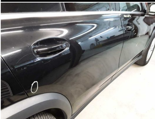
Damage #15: Door - rear right side: Door - Dent / paintcoat dama... - Repair and paint
