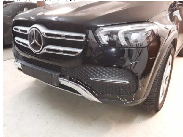
Damage #10: Front bumper: Spoiler - Scratched - Replace
