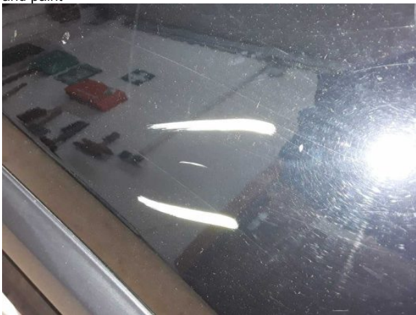
Damage #9: Mudguard - left side: Mudguard - left side - Scratched... Repair and paint
