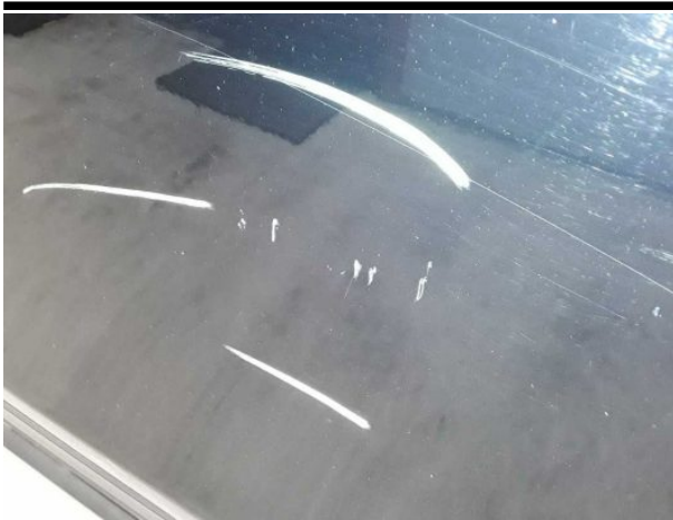
Damage #16: Door - front left side: Door - Dent / paintcoat damage - Repair and paint
