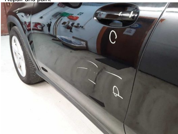
Damage #16: Door - front left side: Door - Dent / paintcoat damage - Repair and paint
