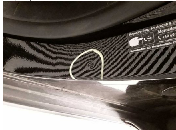
Damage #3: Sill - left side: Sill - dent(s) - Smooth repair work
