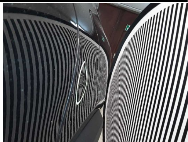
Damage #6: Side panel - rear left side: Side panel - dent(s) - Smooth repair work
