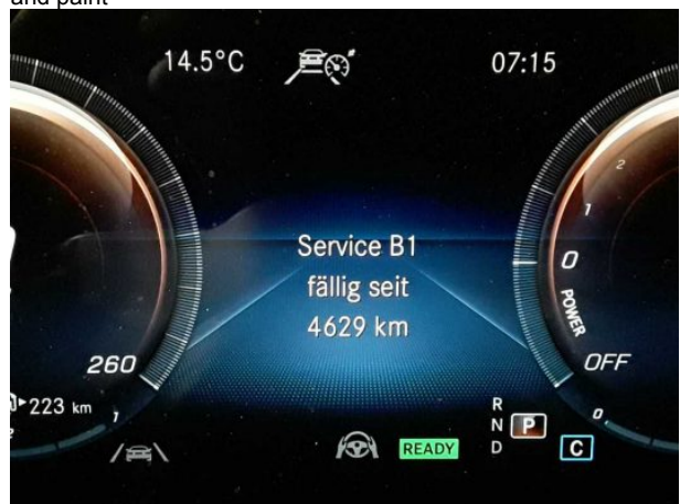
Damage #12: Misc.: Inspection / maintenance - Due - Replace
