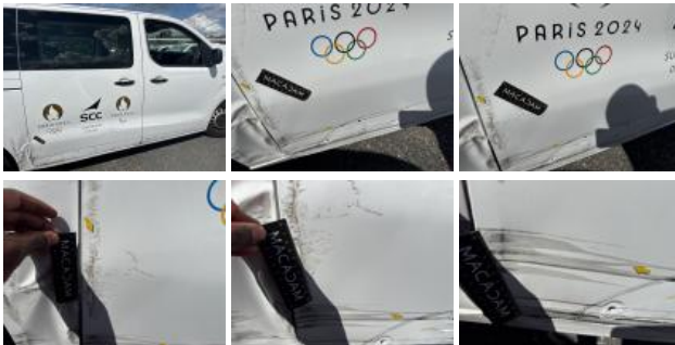
Door trim RR, Missing, Replace
