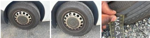
Wheel cover RL, Missing, Replace
