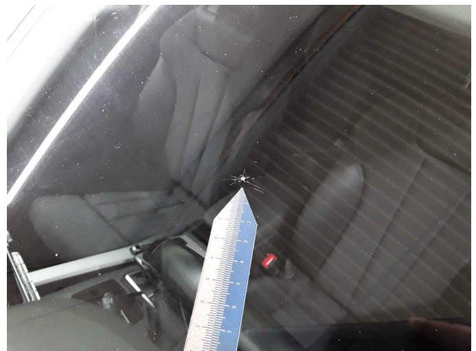
Damage 7: Vehicle glazing: Windscreen - Stone chips - Replace
