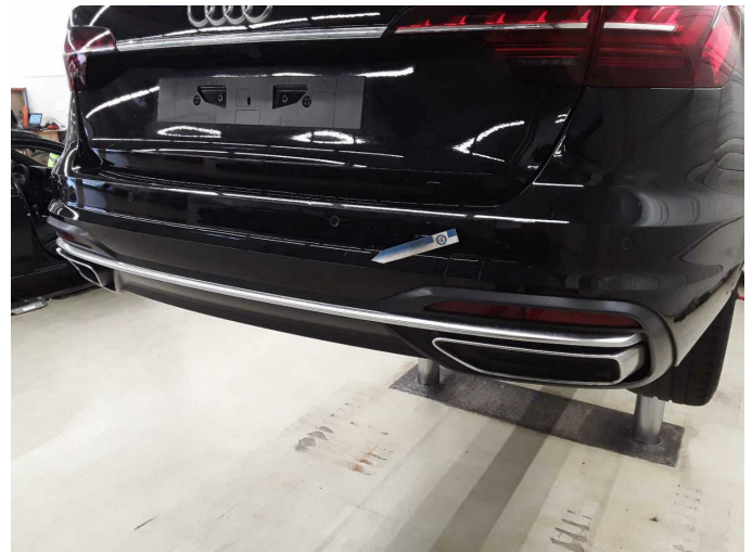
Damage 3: Rear bumper: Rear bumper - Scratch(es) - Repair and paint
