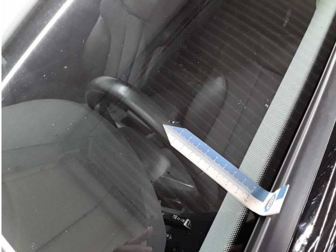
Damage 7: Vehicle glazing: Windscreen - Stone chips - Replace
