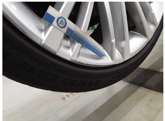
Damage 5: Wheel / tyres: Alloy rim - rear right side - Scratched - Replace
