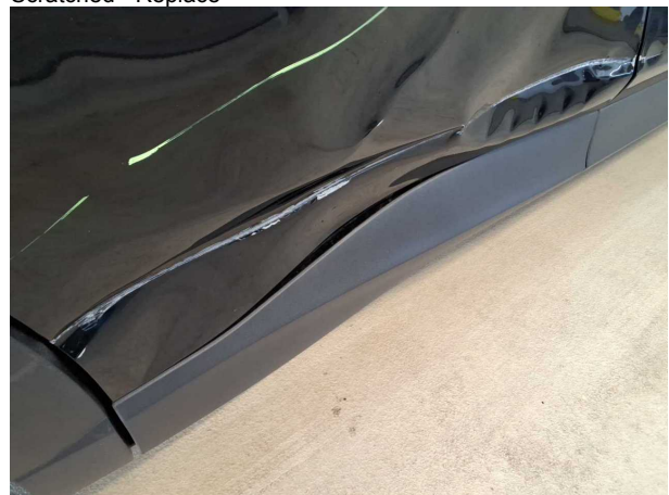
Damage #6: Door - rear right side: Brightware - lower - Scratched - Replace
