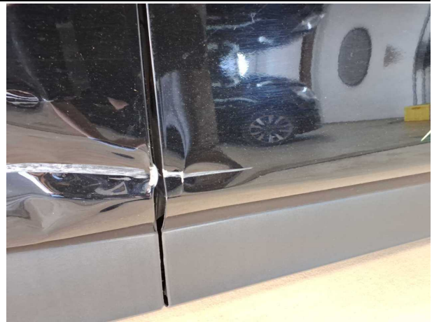
Damage #8: Door - front right side: Door - Dent / paintcoat damage - Replace
