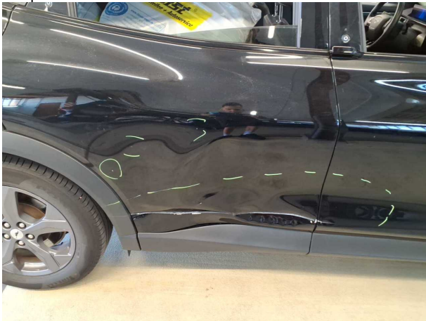
Damage #9: Door - rear right side: Door - Dent / paintcoat damage - Replace
