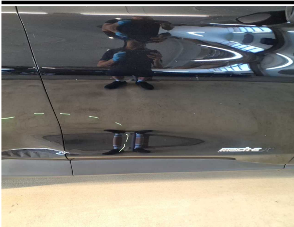
Damage #8: Door - front right side: Door - Dent / paintcoat damage - Replace
