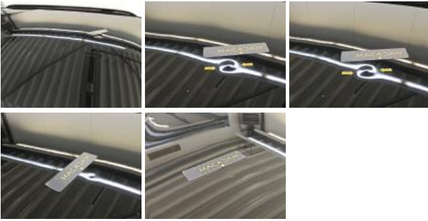
Roof, Dent(s), Repair and paint (complete)
