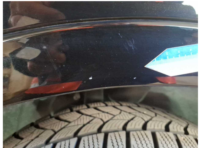
Damage 4: Mudguard - right side: Wheel well extension - Scratched - Smart repair
