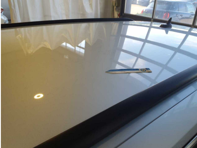
Damage 7: Roof: Roof - Scratch(es) - Paint
