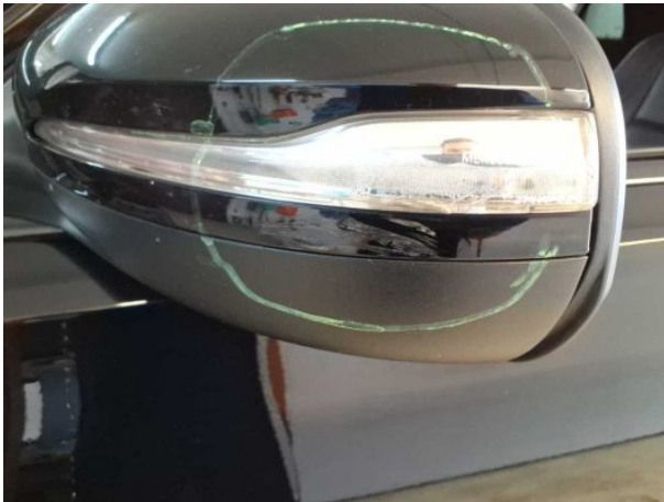
Damage #8: Wing mirror - left side: Cap - Scratched - Smart repair
