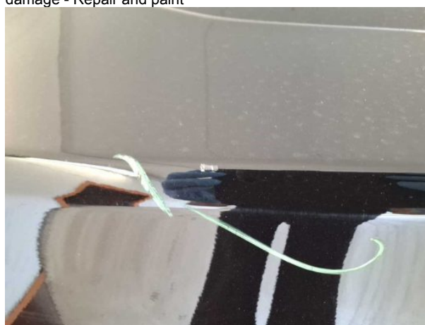
Damage #15: Boot lid / rear door: Boot lid - Dent / paintcoat damage - Repair and paint
