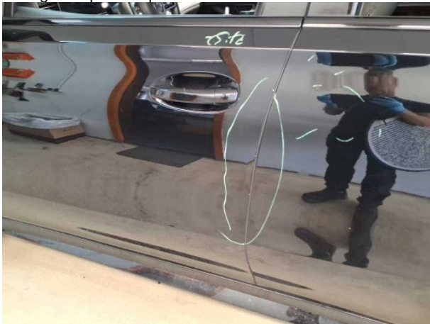
Damage #16: Door - front left side: Door - Dent / paintcoat damage - Replace
