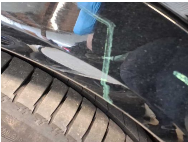
Damage #9: Side panel - rear right side: Wheel well extension - Scratched - Smart repair
