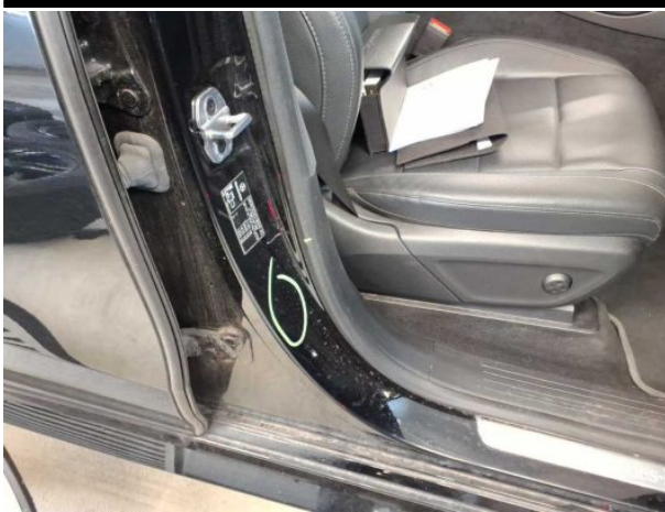
Damage #7: Sill - right side: Sill - dent(s) - Smooth repair work
