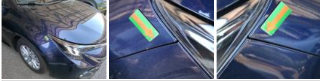
Door RR, Dent(s), Repair and paint (complete)
