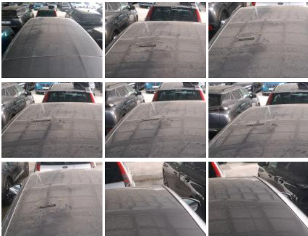
Roof, Dent(s), Repair and paint (complete)
