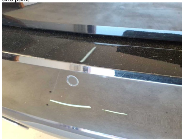
Damage #11: Rear bumper: Rear bumper - Scratched - Repair and paint
