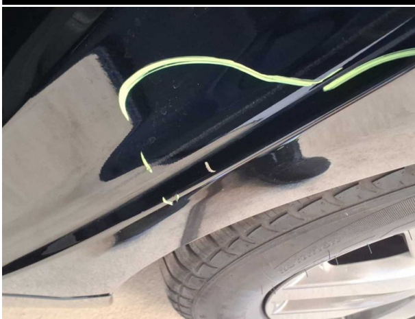
Damage #6: Side panel - rear left side: Sill - Scratched - Smart repair
