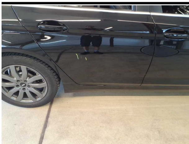
Damage #10: Door - rear right side: Door - Scratch(es) - Repair and paint
