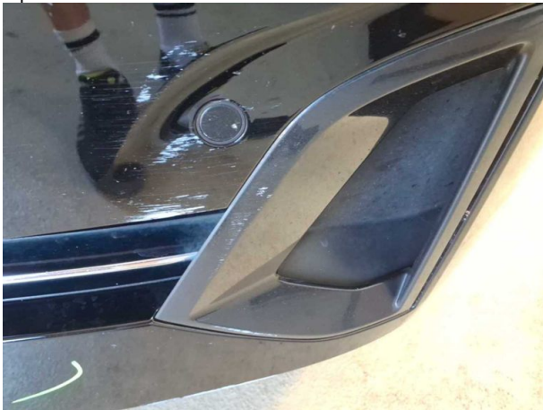
Damage #7: Front bumper: Air-inlet grille - Damaged - Replace
