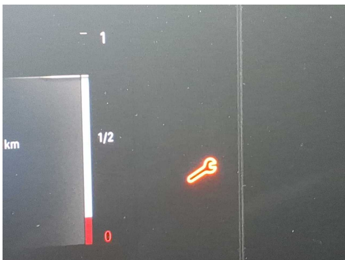
Damage 2: Misc.: Inspection / maintenance - Due - Perform diagnosis
