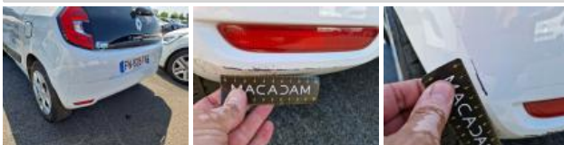
Bodywork, Glue residues, Remove lettering
