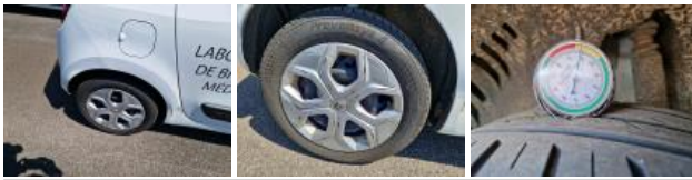
Tyre RL, Out of tolerance, Replace
