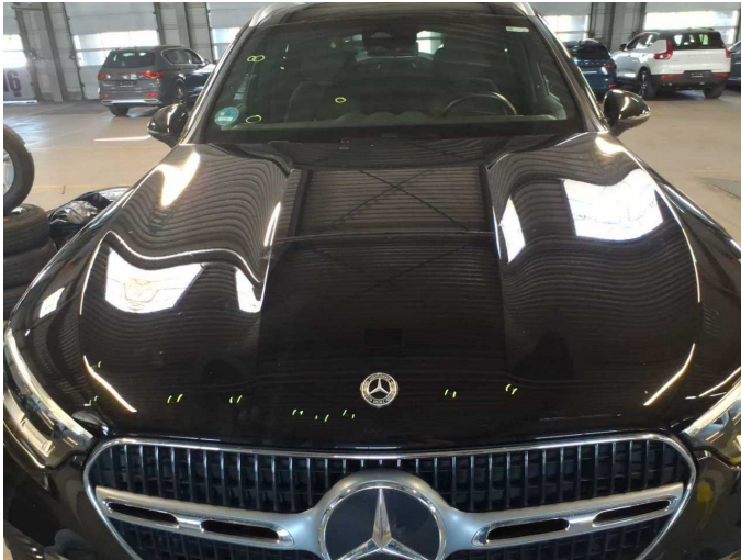
Damage 5: Bonnet: Bonnet - Stone chips - Paint
