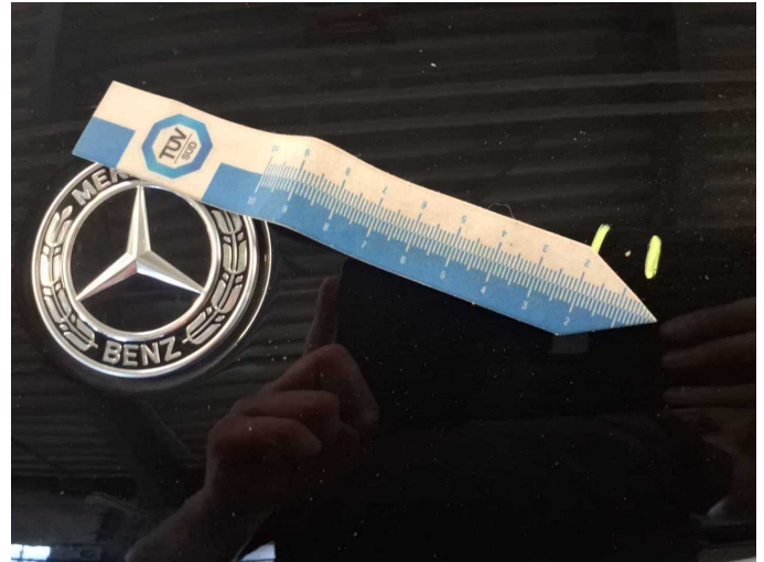
Damage 5: Bonnet: Bonnet - Stone chips - Paint
