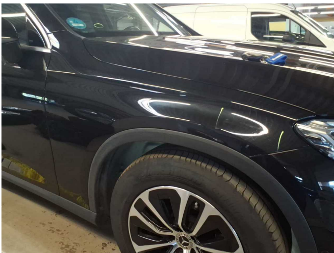
Damage 4: Mudguard - right side: Mudguard - right side (Klarlack milchig + Dellen) - Unprofessionally repaired - Paint
