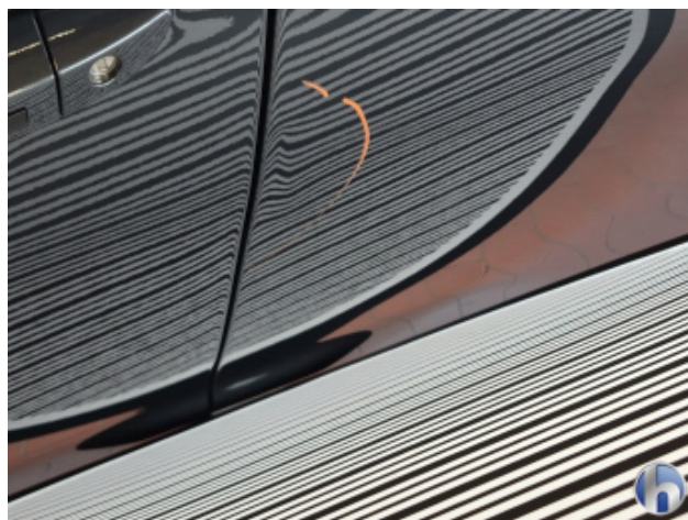
4. Tür Hinten - Links 1 Delle - Sanft Instandsetzen
