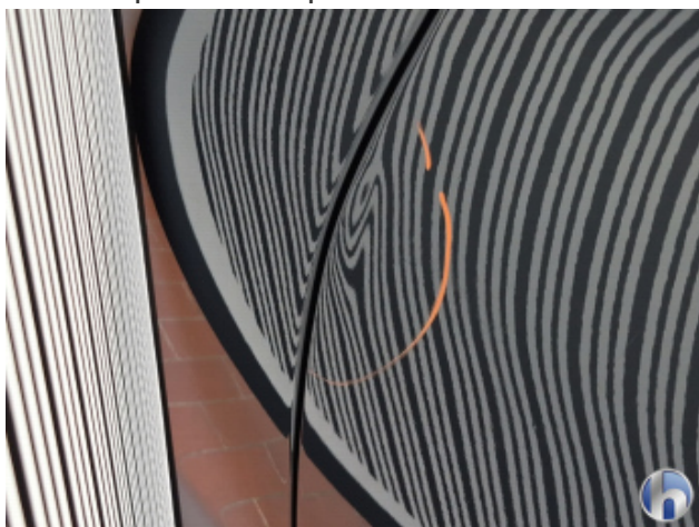
4. Tür Hinten - Links 1 Delle - Sanft Instandsetzen
