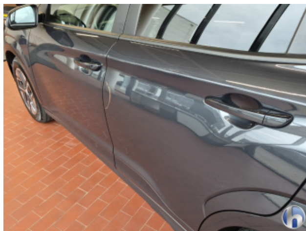
4. Tür Hinten - Links 1 Delle - Sanft Instandsetzen
