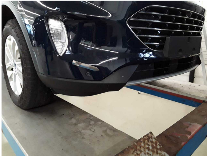
Damage 5: Front bumper: Bumper with Parktronic - Scratch(es) - Paint
