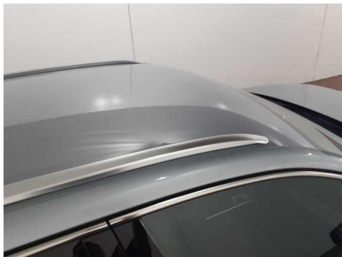
Damage 5: Roof: Roof - dent(s) - Smart repair
