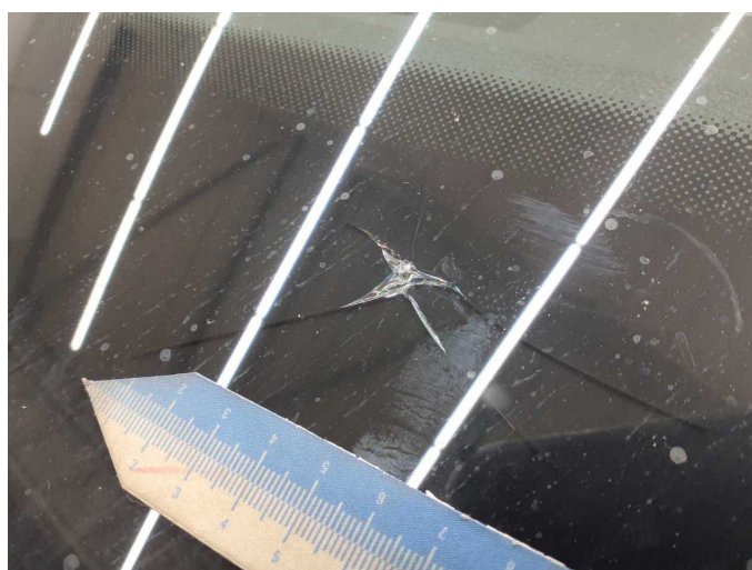
Damage 7: Vehicle glazing: Windscreen - Broken / torn - Replace
