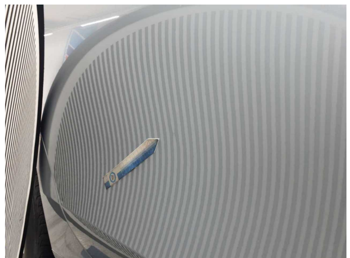
Damage 1: Door - rear right side: Door - dent(s) - Smart repair
