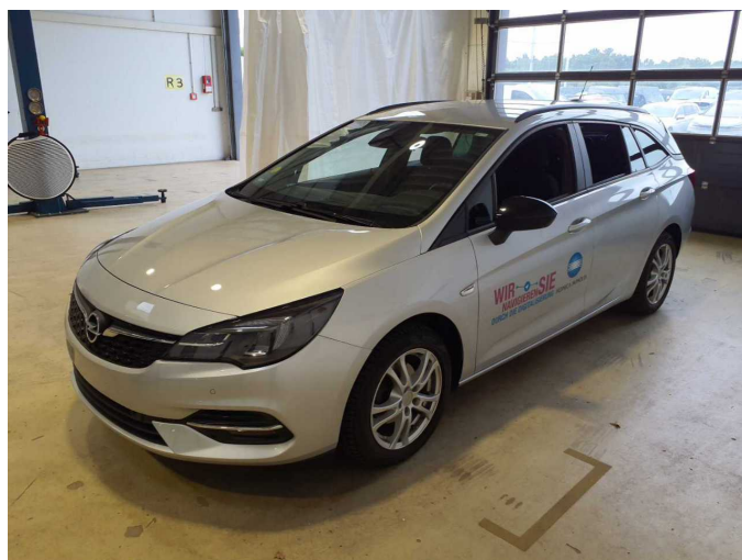
Damage 3: Body: Body - Glued / labelled - De-glue / neutralise
