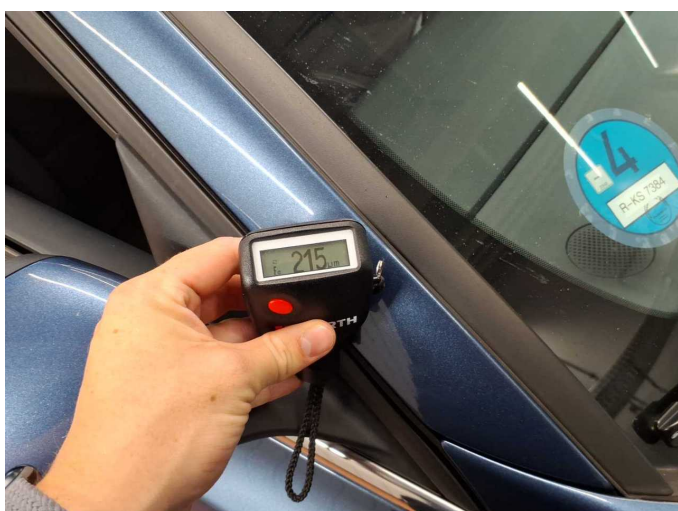
Repainting 1: Roof rail - right side
