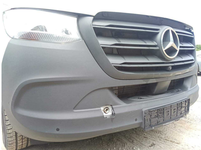
Damage 3: Front bumper: Front bumper - Scratched - Replace
