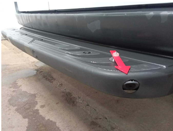
Damage 2: Rear bumper: Parking sensors - right side - Broken / torn - Replace
