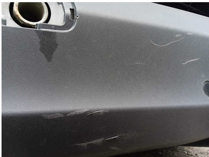
Damage 3: Front bumper: Front bumper - Scratched - Replace
