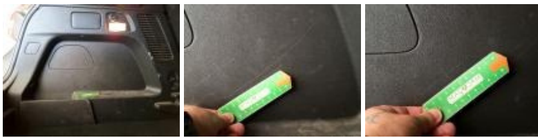
Garnit zone de chargement, Griffe(s), Acceptable
