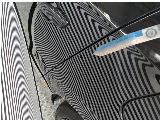
Damage 9: Side panel - rear left side: Side panel (Unterhalb Kante.) - Dent / paintcoat damage - Repair and paint
