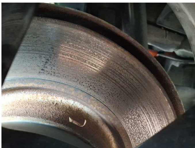
Damage 8: Braking system: Brake discs and pads - rear (Tragbild mangelhaft. Riefen.) - Corrosion - Replace
