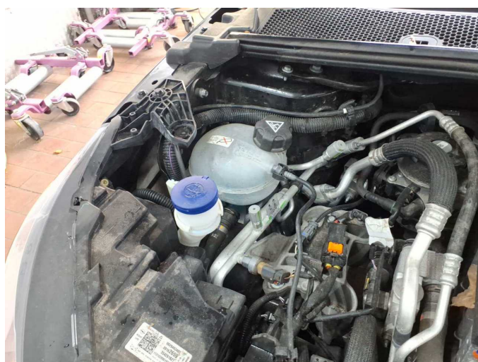
Damage 2: Engine cooling: Coolant (Unter Minimum. Werkstattprüfung erf.) - Specify findings - Diagnosed and repair if necessary
