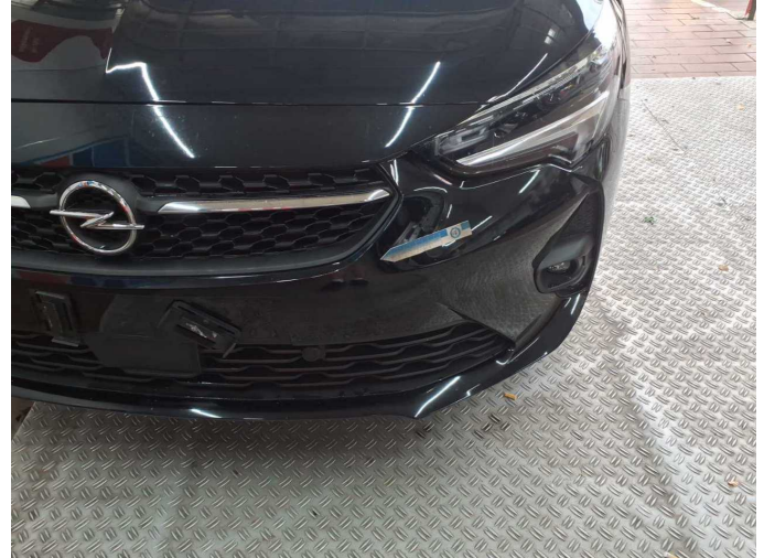
Damage 10: Front bumper: Front bumper - Scratch(es) - Repair and paint
