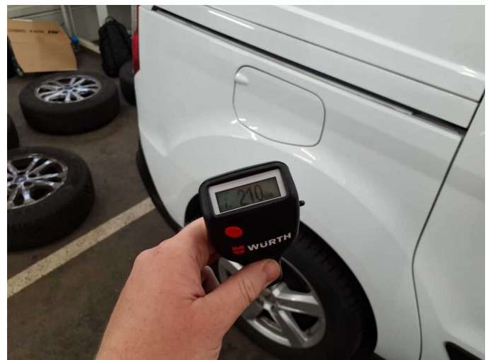
Repainting 2: Side panel - rear right side
