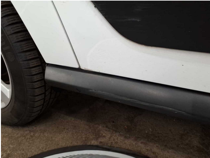
Damage 8: Sliding door, right: Sliding door (+Leiste erneuern) - Dent / paintcoat damage - Repair and paint
