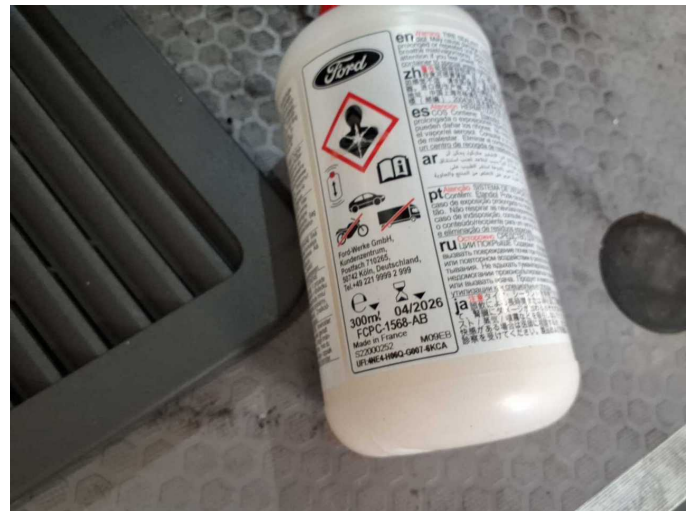
Damage 3: Equipment: Tirefit filler - Expired - Replace
