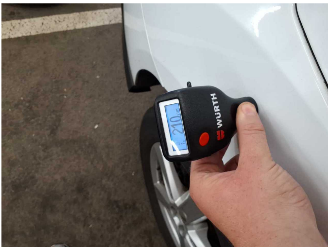
Repainting 2: Side panel - rear right side
