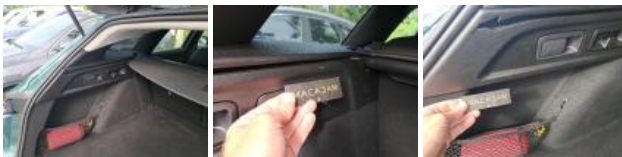
Internal boot lining R, Scratch(es), Acceptable
