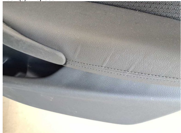
Damage #3: Trim / covers: Door trim - rear right side (Arملهne) - dent(s) - Replace
