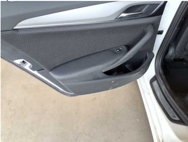
Damage #2: Trim / covers: Door trim - rear left side (Arملهne) - dent(s) - Replace
