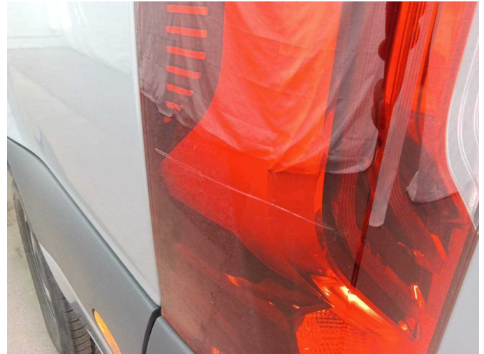
Damage 6: Tail light: Tail lamp - left side - Scratch(es) - Replace
