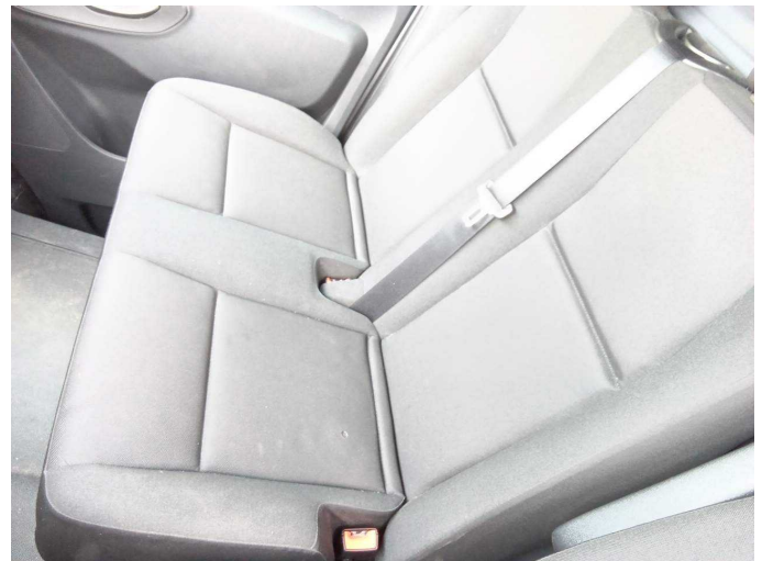
Damage 7: Seat - front: Seat cover - right side - Holes - Replace
