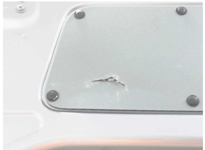
Damage 5: Boot lid / rear door: Trim standard - upper - Holes - Replace
