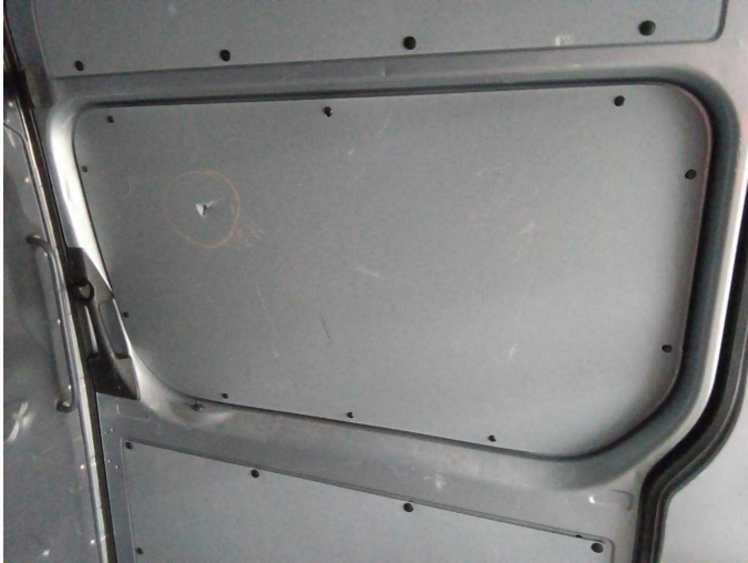
Damage 4: Sliding door, right: Trim - Holes - Replace
