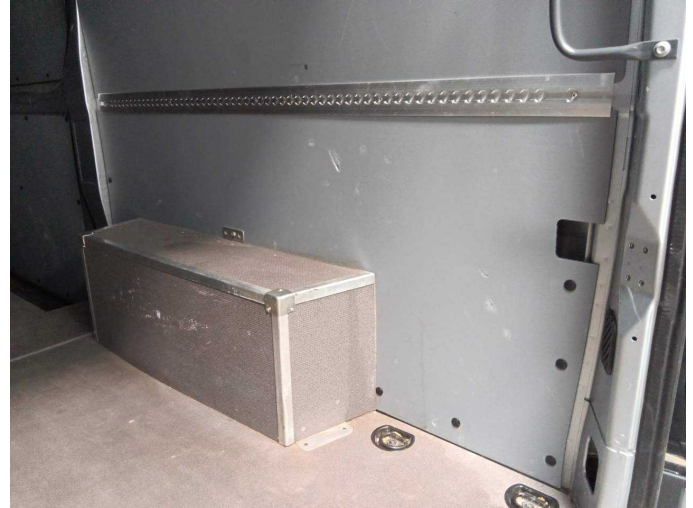
Damage 3: Trim / covers: Cargo area - lining - right side - Holes - Replace
