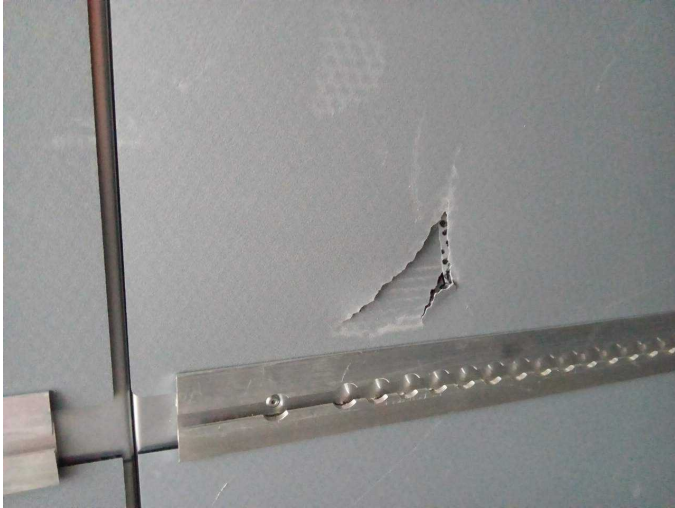
Damage 2: Trim / covers: Cargo area - lining -left side - Holes - Replace
