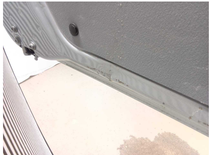
Damage 9: Boot lid / rear door: Rear door - left side - Dent / paintcoat damage - Repair and paint
