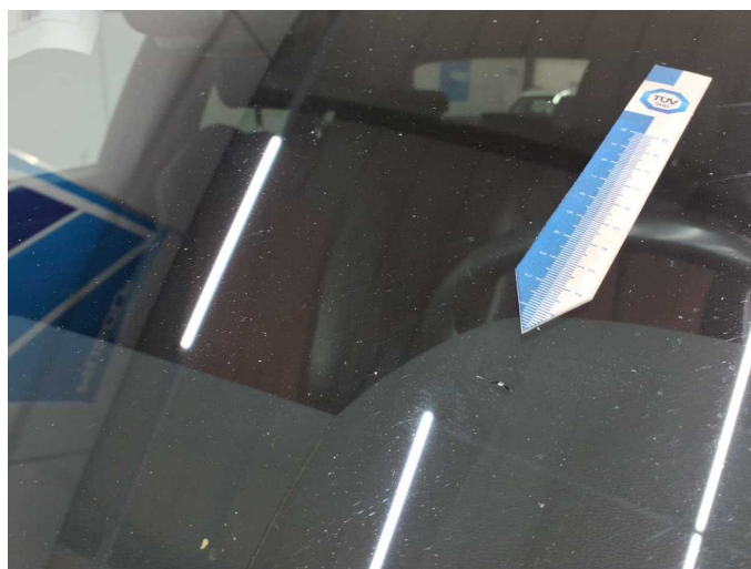
Damage 9: Vehicle glazing: Windscreen - Stone chips - Replace
