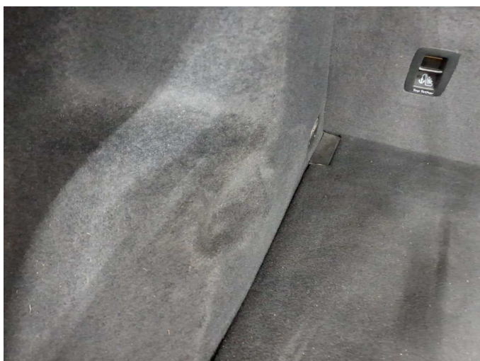
Damage 7: Side panel - rear left side: Interior trim - Deformed - Replace
