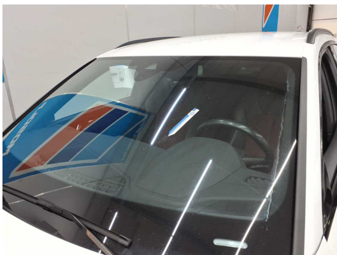
Damage 9: Vehicle glazing: Windscreen - Stone chips - Replace
