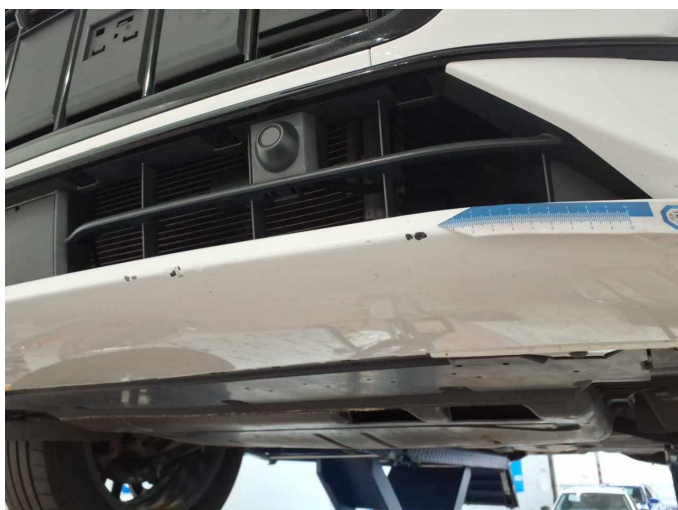
Damage 4: Front bumper: Spoiler - Scratch(es) - Smart repair
