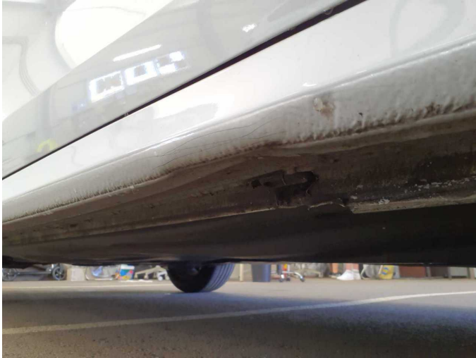
Damage 6: Sill - right side: Sill - Deformed - Repair and paint
