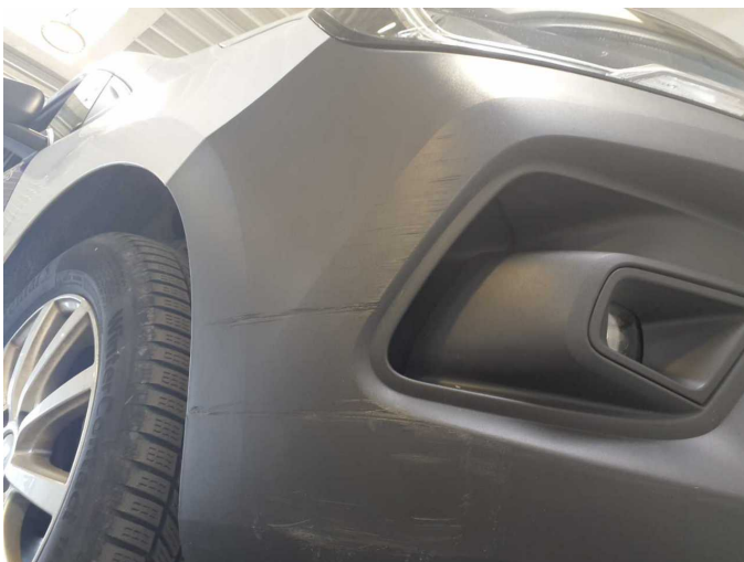
Damage 9: Front bumper: Front bumper (unpainted) (inkl. Schutzleiste) - Scratch(es) - Replace
