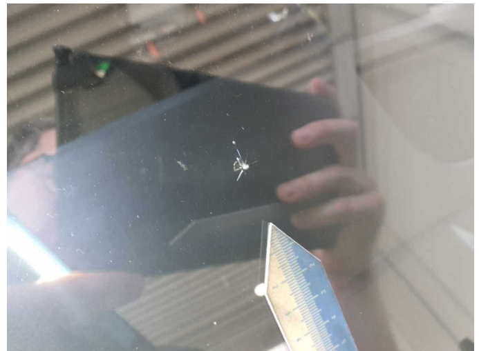
Damage 10: Vehicle glazing: Windscreen - Stone chips - Replace
