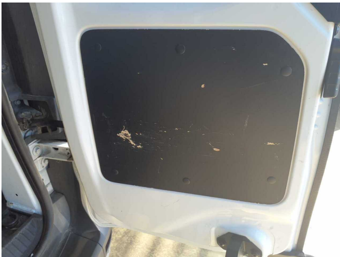
Damage 3: Boot lid / rear door: Trim rear door - hard fibre - lower - Broken / torn - Replace
