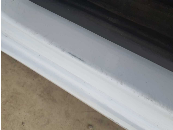
Wear and tear 3: Sill - left side: Sill - Scratch(es) - No deduction
