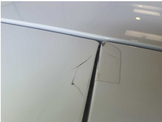
Damage 8: Boot lid / rear door: Rear door - left side - Dent / paintcoat damage - Paint
