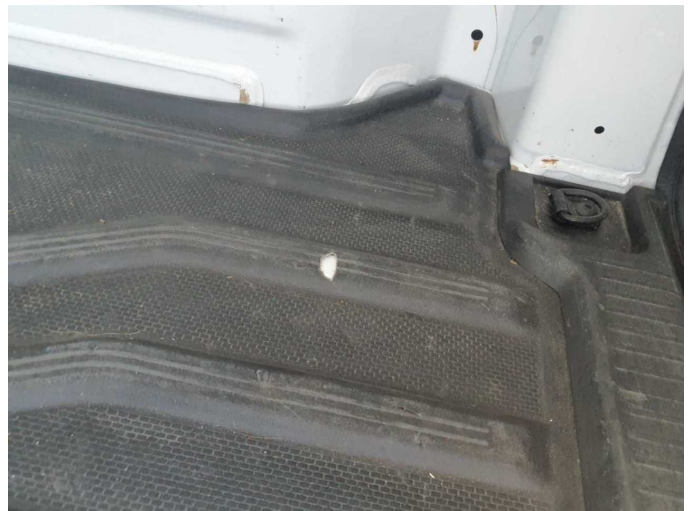
Damage 6: Interior: Cargo area floor - Broken / torn - Replace
