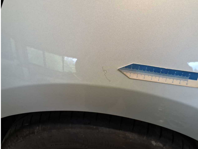
Damage 5: Side panel - rear left side: Side panel - Scratch(es) - Paint
