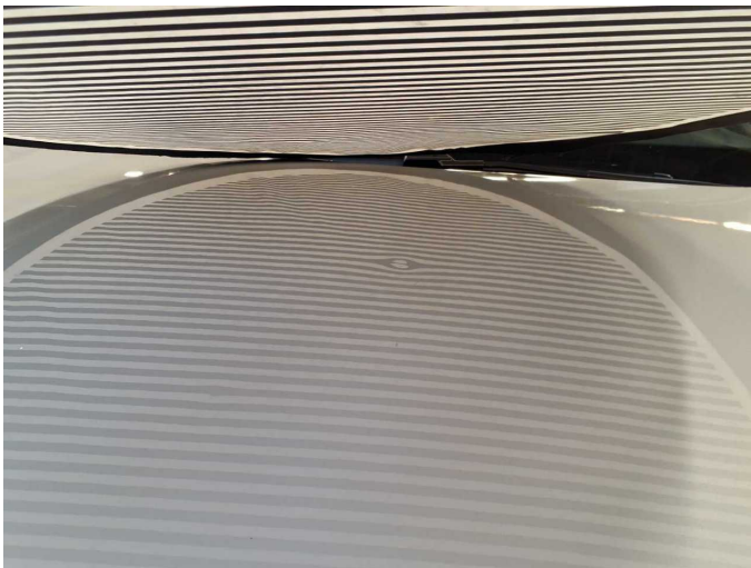
Damage 6: Body: Body - Damage by hail - Smooth repair work
