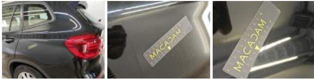
Bumper F, Scratch(es), Repair and paint (complete)
