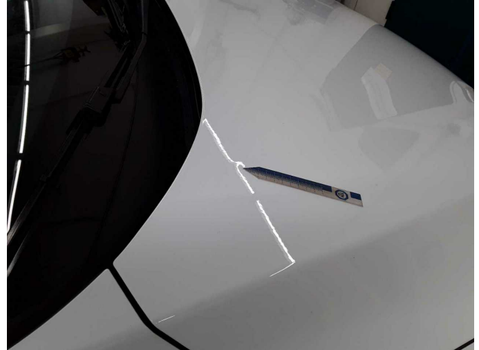
Damage 11: Body: Body (Hagelschaden) - dent(s) - Repair
