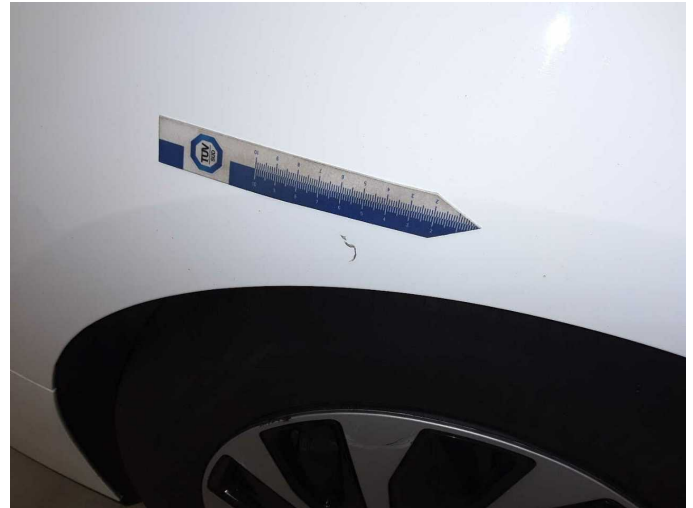
Damage 8: Side panel - rear right side: Side panel - Scratch(es) - Smart repair
