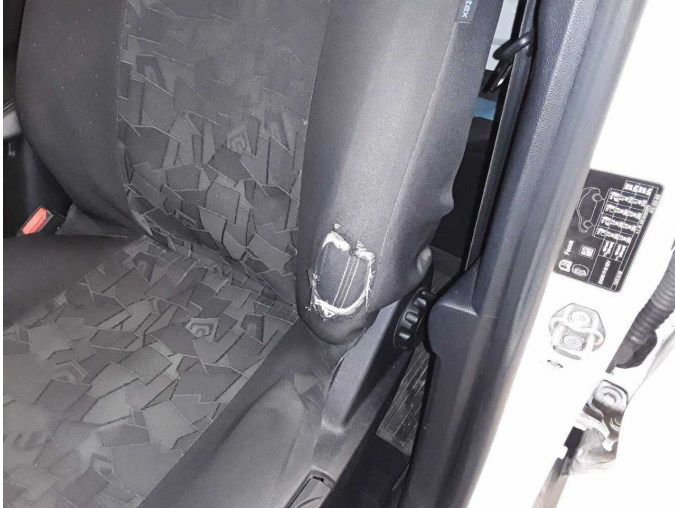
Damage 2: Seat - front: Protective Cover - left side - Broken / torn - Replace
