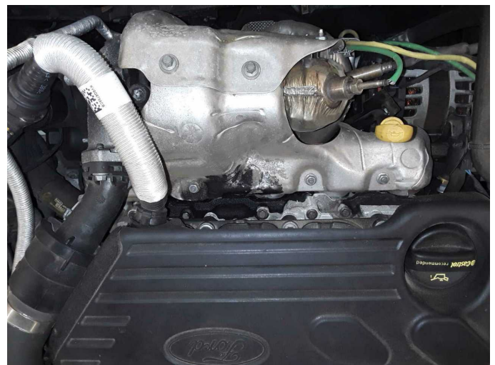
Damage 7: Engine: Engine (Ölspuren erkennbar) - Soiled - Diagnosed and repair if necessary
