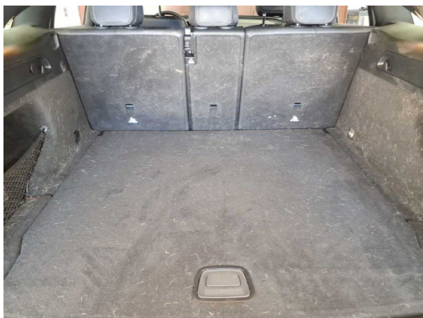
Damage #6: Interior: Interior - Soiled - Clean
