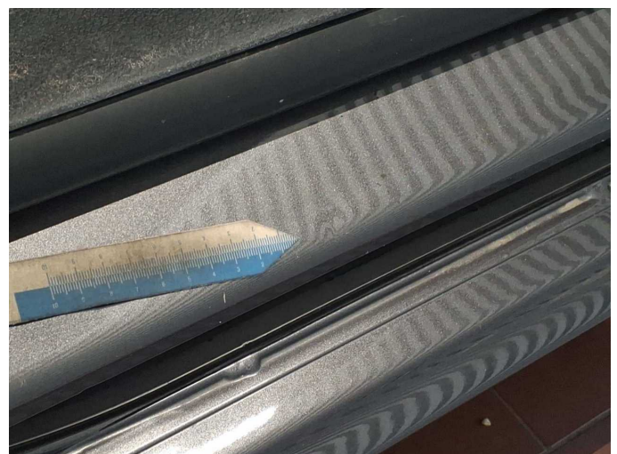
Damage 6: Side panel - rear left side: Sill - dent(s) - Smart repair
