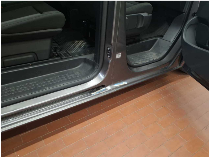
Damage 11: Sill - right side: Sill - Scratch(es) - Smart repair
