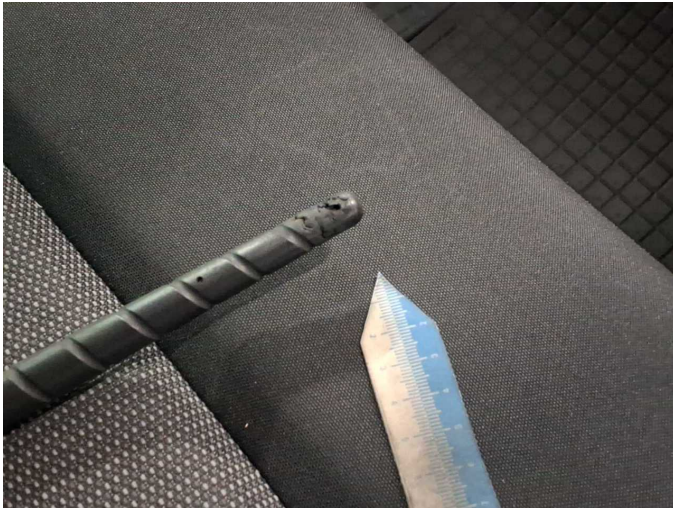
Damage 1: Roof: Stub aerial - Damage caused by marten / rodent - Replace
