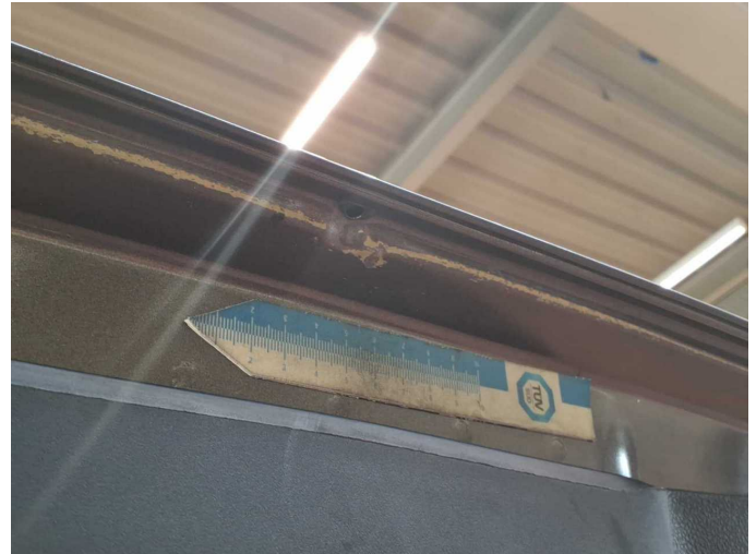
Damage 9: Boot lid / rear door: Boot lid - Scratch(es) - Smart repair
