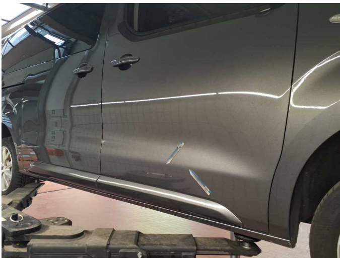
Wear and tear 10: Door - front right side: Door - dent(s) - No deduction
