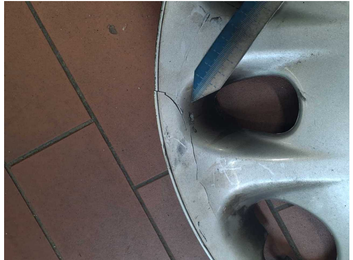
Wear and tear 9: 2nd wheel set: 1 wheel cover (Zubehör) - Broken / torn - No deduction
