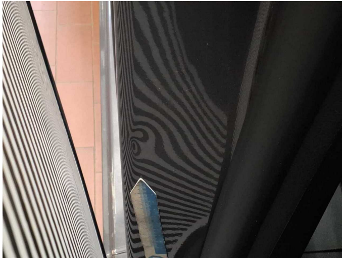
Damage 4: Body: B-pillar - right side - dent(s) - Smooth repair work
