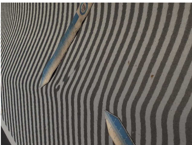
Wear and tear 10: Door - front right side: Door - dent(s) - No deduction
