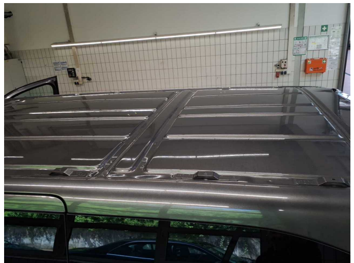
Damage 14: Roof: Roof - Damage by hail - Smooth repair work
