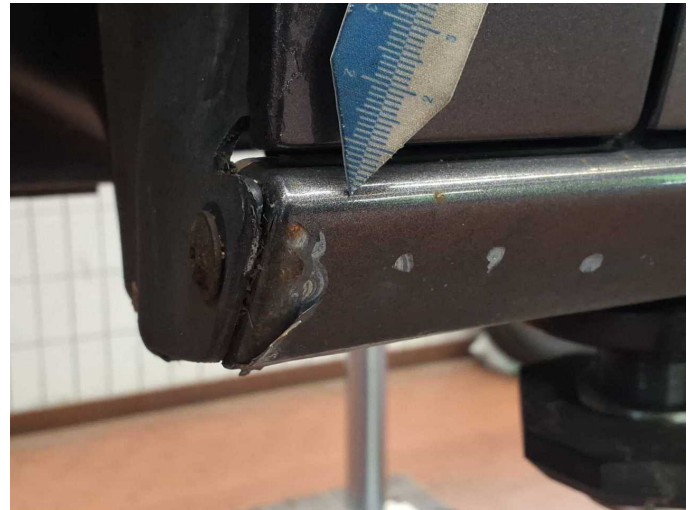
Damage 13: Sill - left side: Sill - Dent / paintcoat damage - Repair and paint
