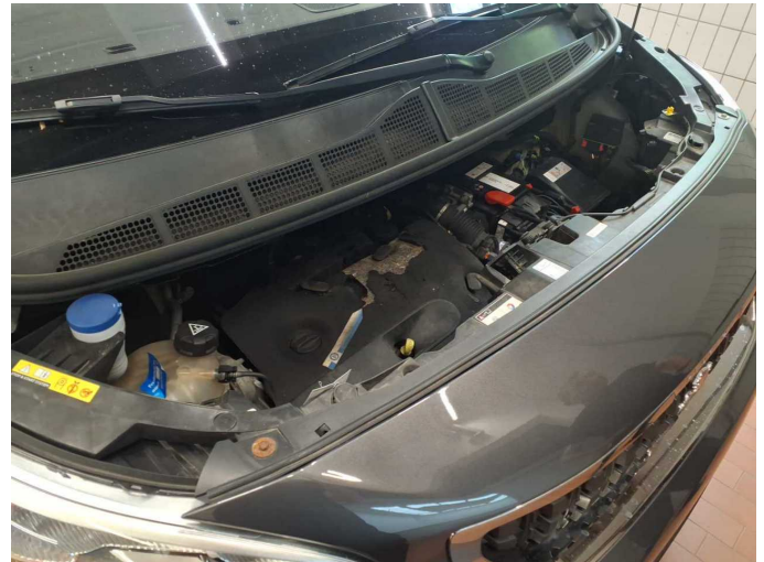
Damage 12: Engine: Engine cover - Damage caused by marten / rodent - Replace
