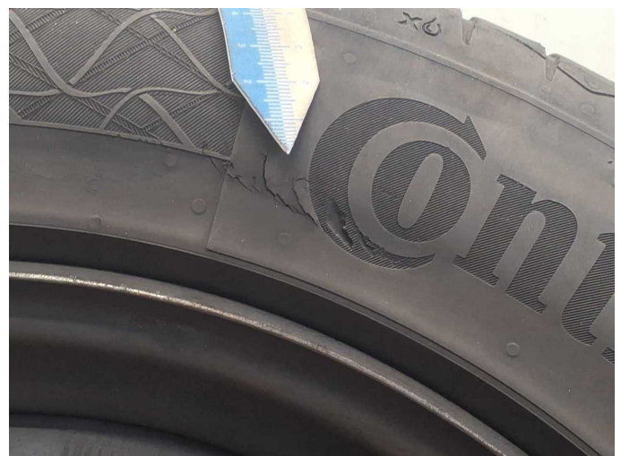
Damage 10: 2nd wheel set: 1 tyre - Broken / torn - Replace
