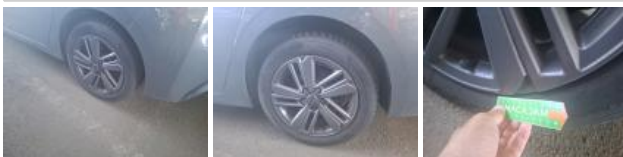
Tyre RL, Out of tolerance, Replace
