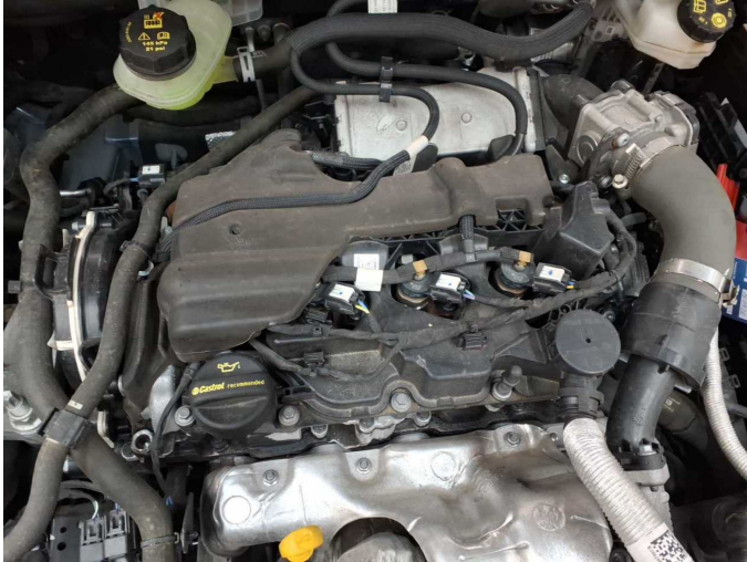
Missing part 1: Engine: Engine cover - Missing - Replace
