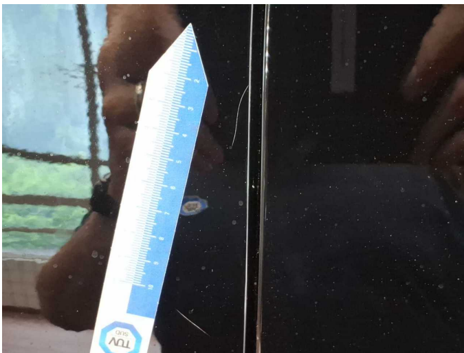
Damage 2: Door - rear left side: Door - Scratch(es) - Smart repair
