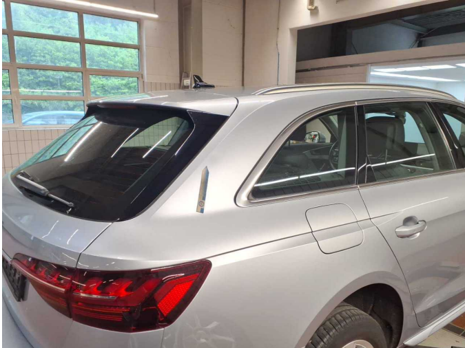
Damage 6: Side panel - rear right side: Side panel (An Kante) - dent(s) - Repair and paint
