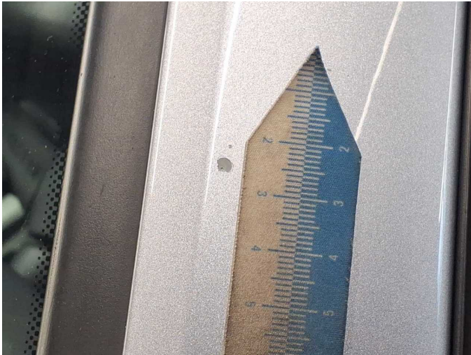
Damage 3: Roof: Roof rail - left side - Stone chips - Smart repair
