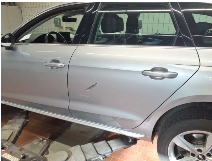
Damage 2: Door - rear left side: Door - dent(s) - Smart repair
