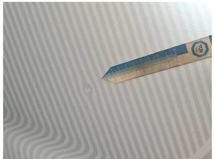
Damage 2: Door - rear left side: Door - dent(s) - Smart repair
