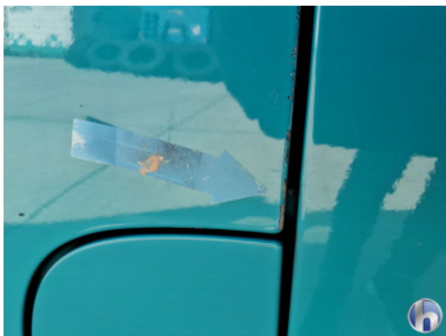
4. Tür Vorne - Links Kratzer - Smart Repair
