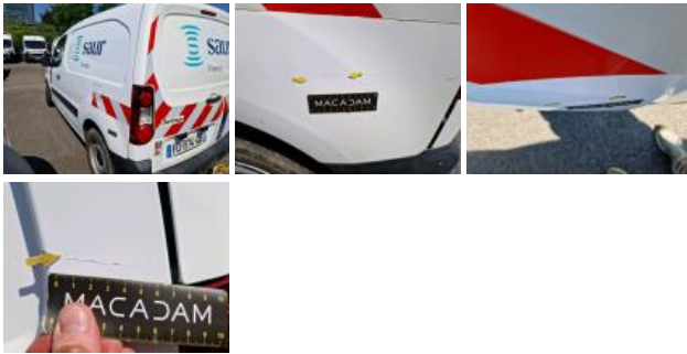
Bumper F, Deformed / Strained, Replace
