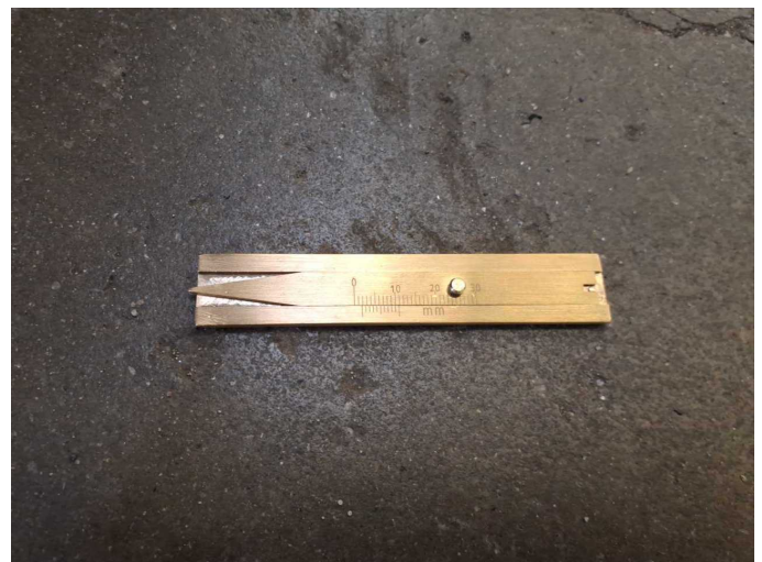
Damage 3: 2nd wheel set: Tyres - complete set (Profiltiefe 2/4mm) - Not admissible - Replace
