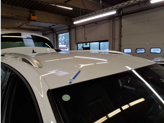
Damage 4: Roof: Roof - Dent / paintcoat damage - Repair and paint
