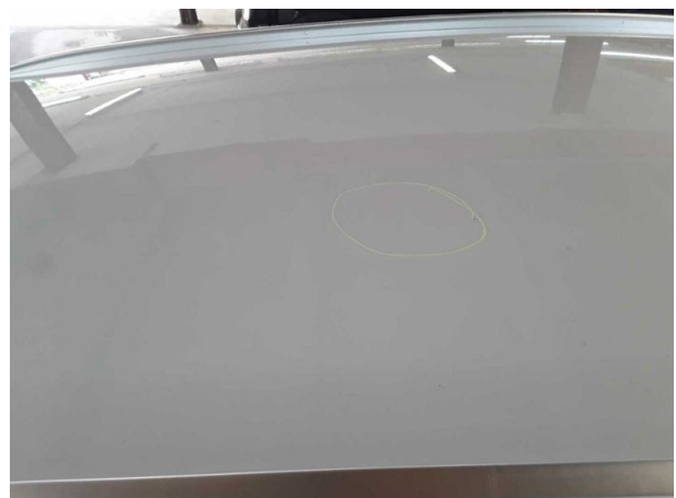
Damage #3: Roof: Roof - dent(s) - Smooth repair work
