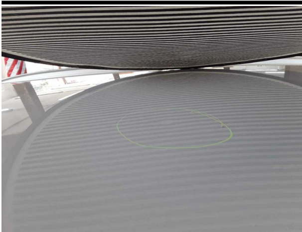
Damage #3: Roof: Roof - dent(s) - Smooth repair work
