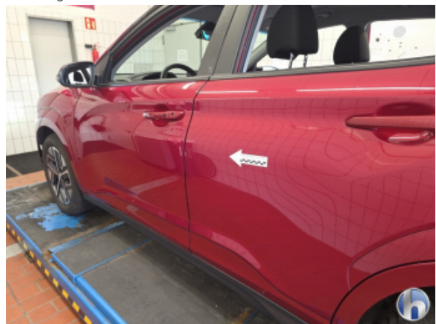
1. Tür Hinten - Links 1 Delle - Sanft Instandsetzen
