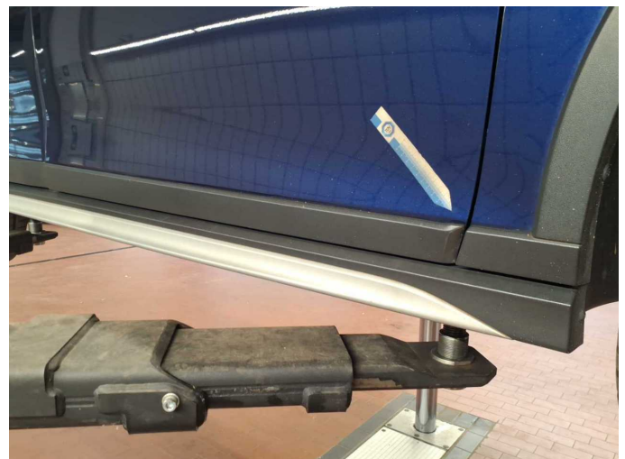
Damage 5: Door - front right side: Brightware - lower - Deformed - Replace
