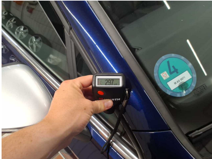
Repainting 1: Roof rail - right side
