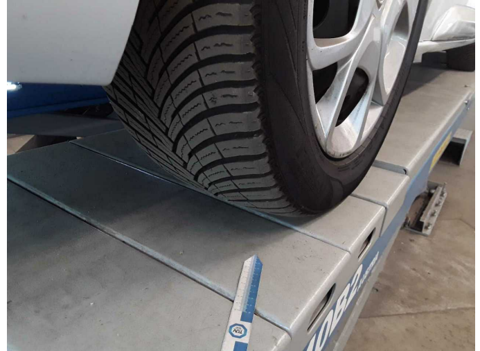
Damage 6: Wheel / tyres: Tyre - front - Worn - Replace
