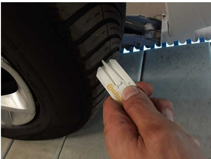
Damage 6: Wheel / tyres: Tyre - front - Worn - Replace
