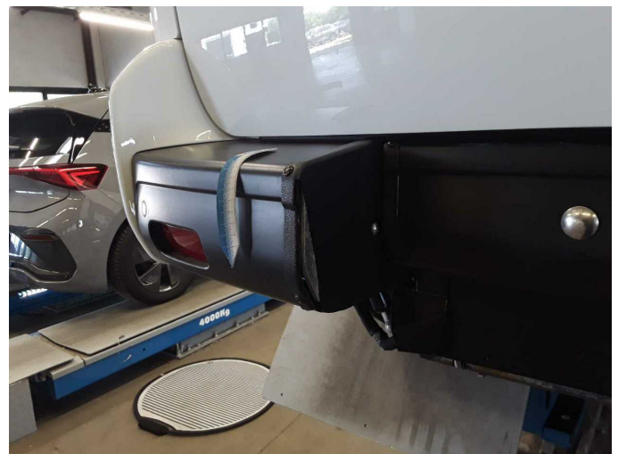
Damage 5: Rear bumper: Rear bumper (Abdeckung, Umbau, Be-Entladespuren) - Damaged - Loss in value
