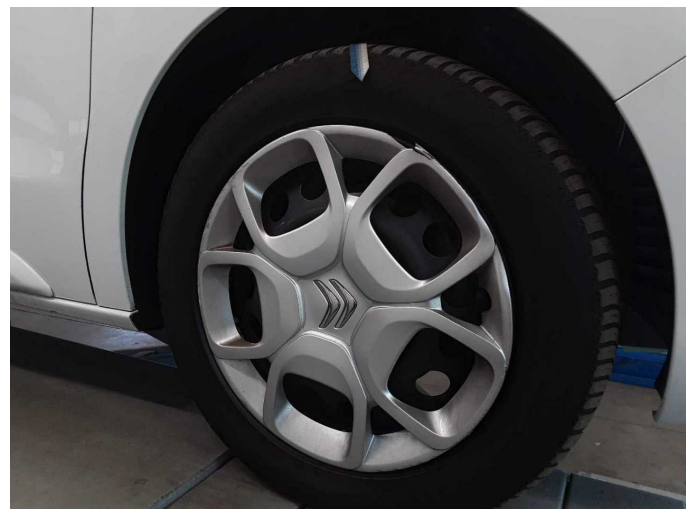
Damage 2: Wheel / tyres: Wheel cover - front right side - Broken / torn - Replace
