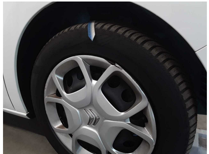
Damage 6: Wheel / tyres: Tyre - front - Worn - Replace
