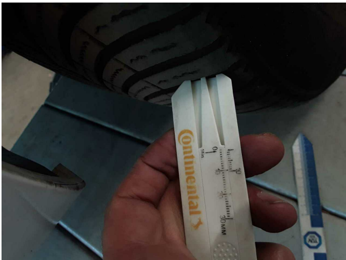
Damage 6: Wheel / tyres: Tyre - front - Worn - Replace
