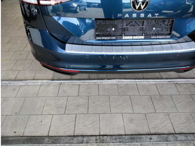
Damage 8: Rear bumper: Rear bumper - Scratch(es) - Paint
