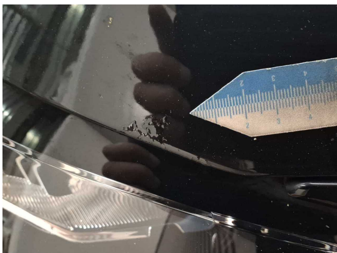
Damage 9: Bonnet: Bonnet - Paint defect - Paint
