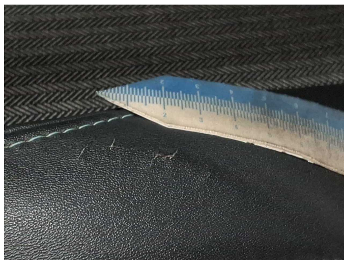
Damage 8: Seat - front: Seat cover - left side - Porous / cracked - Replace
