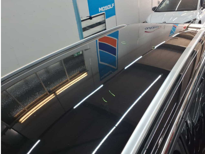
Damage 5: Roof: Roof - dent(s) - Smooth repair work
