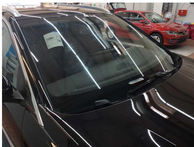
Damage 10: Vehicle glazing: Windscreen - Stone chips - Replace
