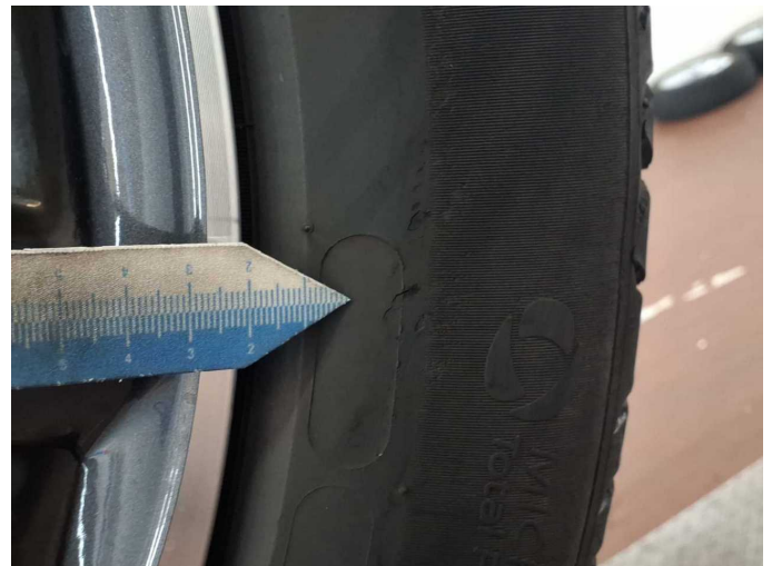
Damage 6: Wheel / tyres: Tyre - front right side - Broken / torn - Replace
