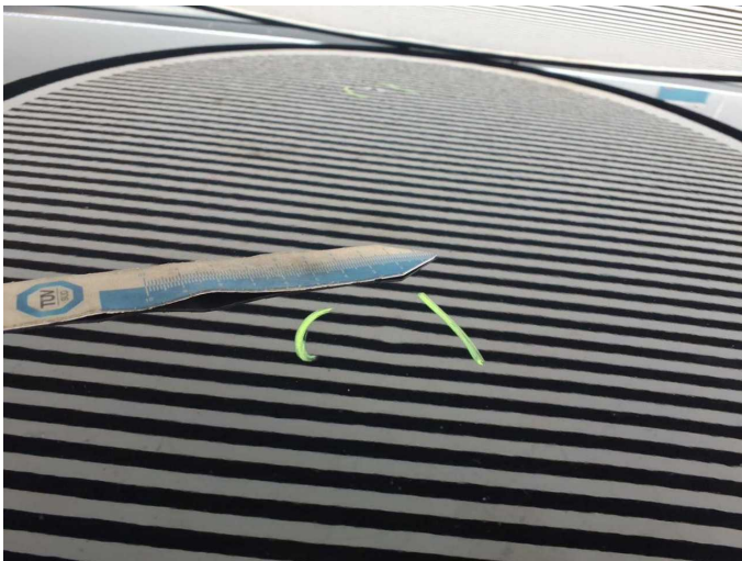
Damage 5: Roof: Roof - dent(s) - Smooth repair work
